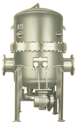
Figure 24 - CUNO™ EF Series Self Cleaning Metal Filters Model MSVR-5, the largest, containing five 7.6" diameter x 24" long cartridges in an ASME code vessel, with fluid flow rates (100 S.S.U.) up to 4700 gpm.
